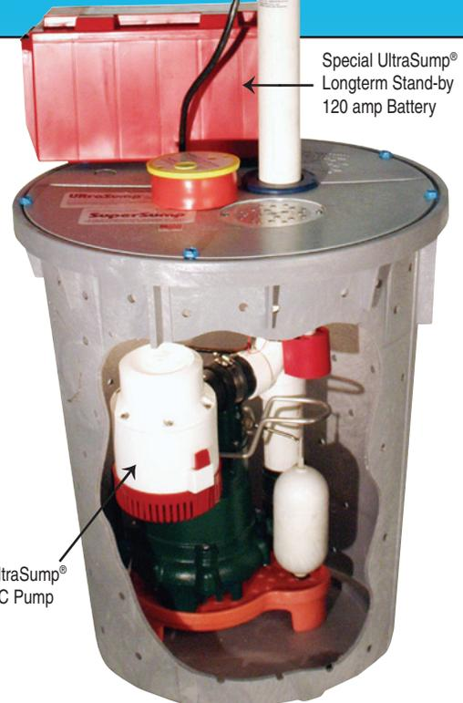
As an addition to your SuperSump®, we recommend a back-up pumping system. The UltraSump® represents the state-of-the-art in battery back-up pumping systems. When added as an option to our SuperSump®, the UltraSump® will turn on automatically if the primary pump fails to operate. The UltraSump® includes a second DC operated pump, a second automatic switching system, a 'smart' charging system, and a high-quality 120 amp battery.
